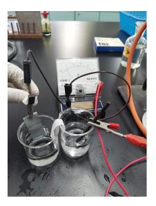
However, we found some problems after doing the experiment which are the low efficiency of the production of hydrogen and low output of voltage. Therefore we decided to use another method to break down carbon dioxide, electrolysis.
